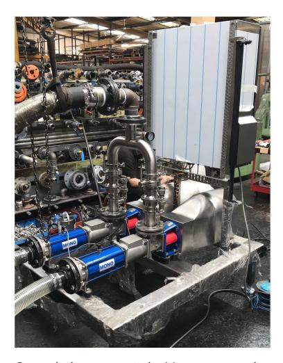
Our solution was a twin Mono progressive cavity unit with seal flushing, controlled by a Vega radar level sensor. All component parts in 316 stainless steel. The sensor, via our control panel allows for duty rotation and parallel variable speed starts and stops depending on the current flow rate.
